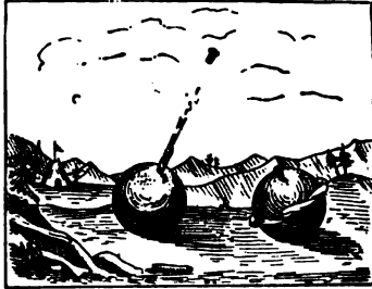
FIG. 123.—EXPANSIVE FORCE OF ICE.
